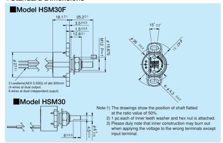
Note: The difference between HSM30F and HSM30 is with or without flange only. The following performances are the same.
